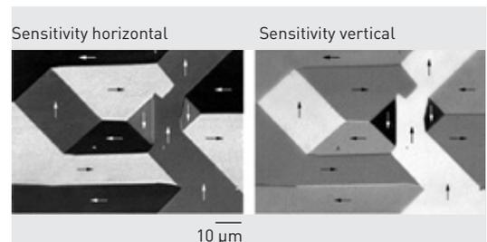
**$\text{Ni}_{81}\text{Fe}_{19}$  stripe:** Magnetic domain structure in 500 nm width nano-wire
